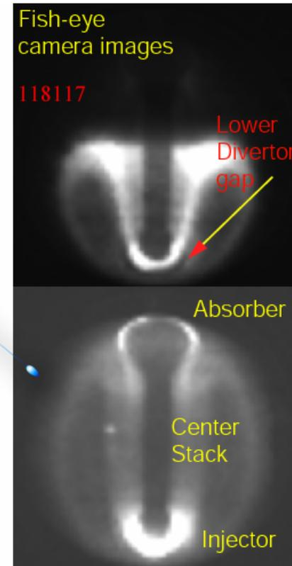
Expect axisymmetric reconnection at the injector to result in formation of closed flux surfaces
