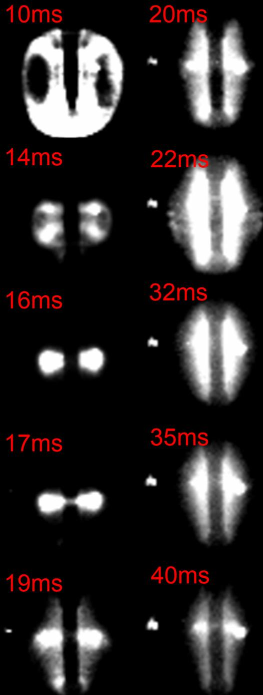
Until  $t=19\text{ms}$ , the plasma continues to shrink in size along the CS. Then for the subsequent 15ms, it becomes diffuse and spreads along the center column. As seen at 22ms, there are diffuse structures indicating field lines at larger major radius near the mid-plane, Then starting at about 35ms, the elongation shrinks and it once again becomes a small more discharge localized to the mid-plane for the subsequent 200 to 400ms.
