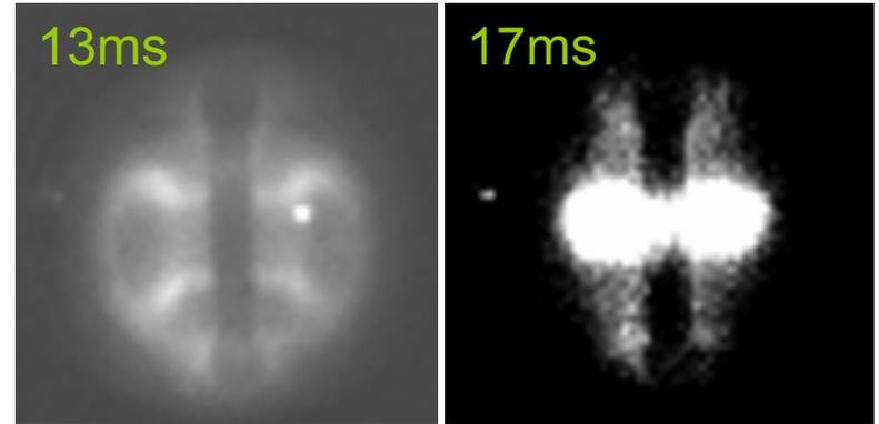
Good Thomson  $T_e$  and  $n_e$  profiles obtained when fast camera shows presence of closed flux region
